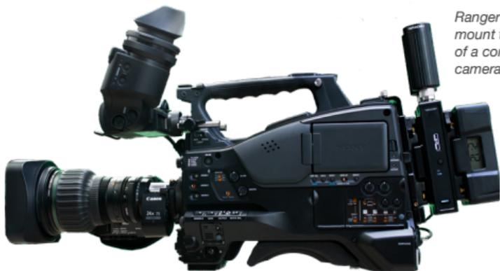
*Ranger transmitters mount to the back of a compatible camera*
