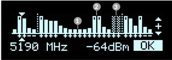
Frequencies are represented by bars; the higher the bar, the more congested that frequency is. Bars without a dot (1) indicate the frequency is not as saturated and can be used. Bars with a dot (2) indicate the frequency is too saturated to connect to. Faded bars (3) represent a frequency that is unavailable for use due to restrictions in particular regions.
